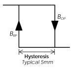
increases enough that it crosses the rising trigger point  $(B_{op})$  the sensor triggers. As the magnet is then moved away from the sensor, the magnetic field strength falls but the sensor remains in the triggered state until the field falls below the falling trigger level  $(B_{RP})$ . The difference between these two points is the hysteresis.
