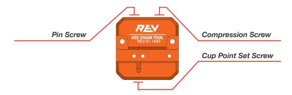
Figure 1: #25 Chain Break Tool Diagram
